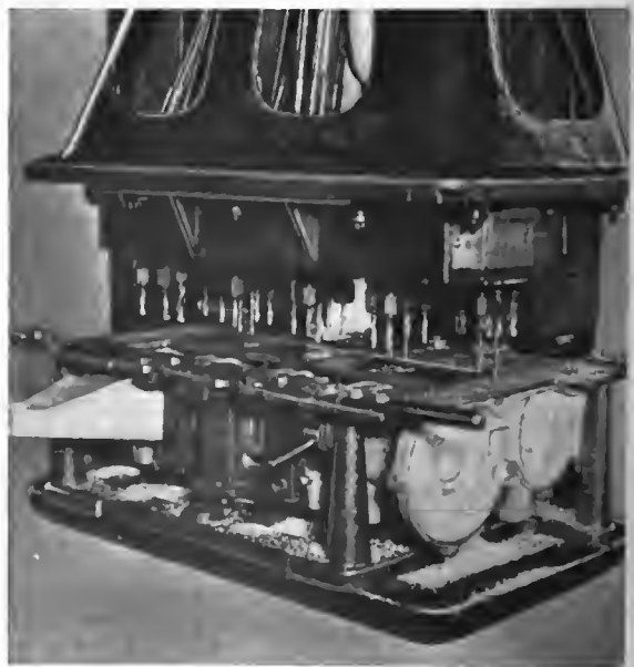
C—Crank Case on the Platen of a Thirty-two Spindle Drill Using a Jigging Fixture Having All the Holes Drilled at One Time.
